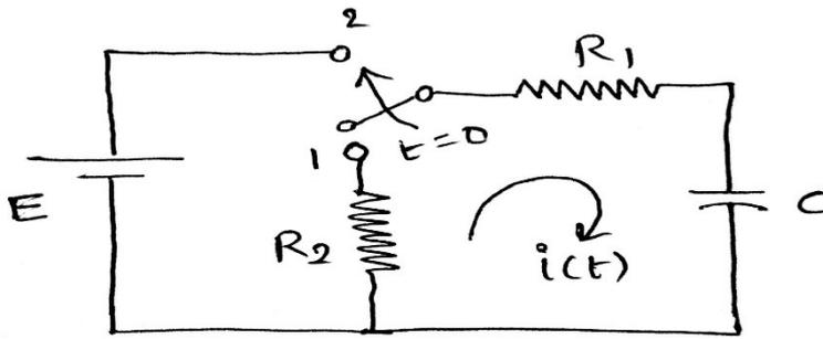
3.a) Draw the pole zero diagram for the given network function and obtain the time domain response  $i(t)$ .
