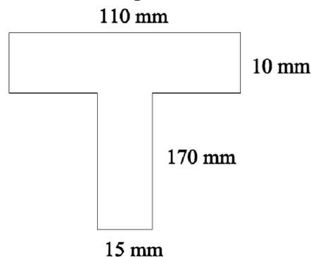
b) Determine the Centroid of the shaded area as shown in fig with respect to x and y axes. All dimensions are in mm.
